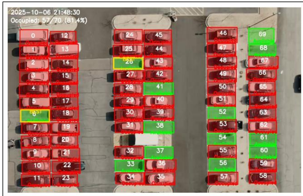
Fig. 2. Flask-based Web Dashboard Interface showing real-time parking status.
