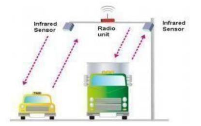
Fig.2. Vehicle detection
