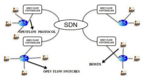
Fig.3. SDN Design architecture
