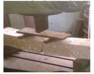
Fig. Determination of Flexural strength of prism Compressive Strength,  $C = \frac{1}{A}$ Where, P= load in Newton A= area of cross section of cube in  $mm^2$ 2PSplitting tensile strength,  $S = \frac{1}{\pi X l X d}$ Where, P= load in Newton l= length of cylinder in mm i.e. 300mm d= diameter of cylinder in mm i.e. 150mm
