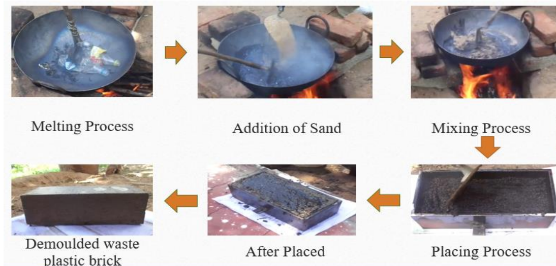
Fig 4 Preparing steps of waste plastic sand bricks
