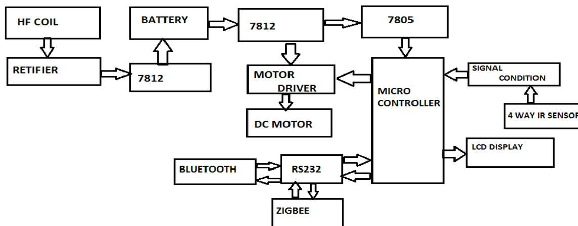
Fig 3.1 Autonomous electrical vehicle with wireless charging
